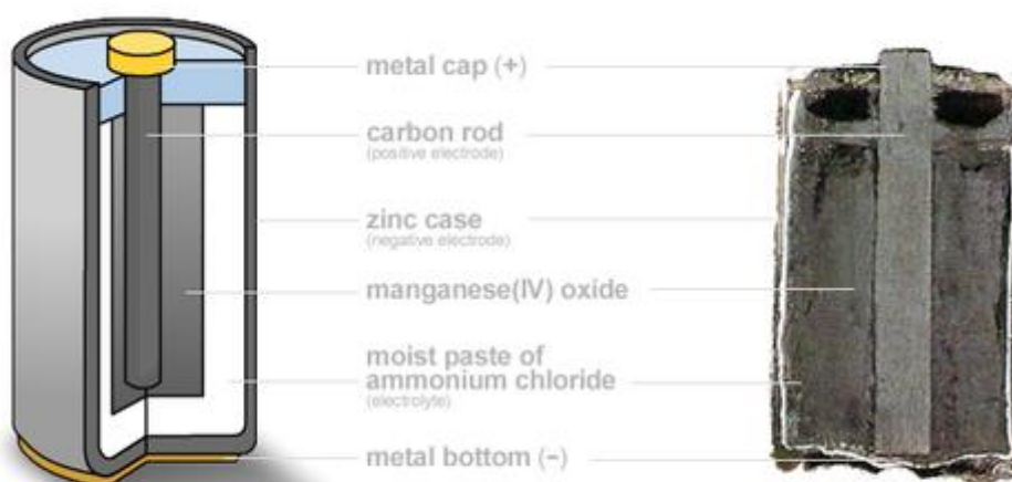
Zinc-Carbon battery ( not 'alkaline')
